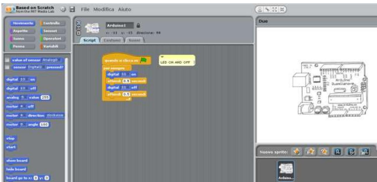
Fig. 4. The S4A code for switching on and off a LED.
